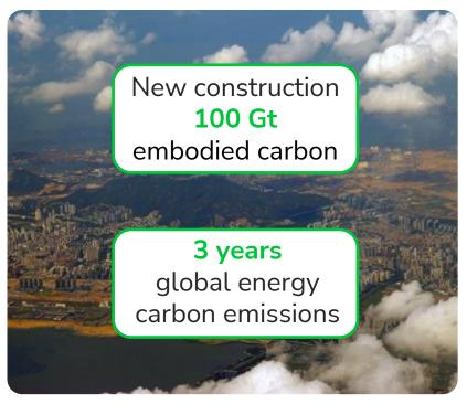
Embodied carbon = CO2e from manufacturing, transporting, installing, replacing and disposing of materials
